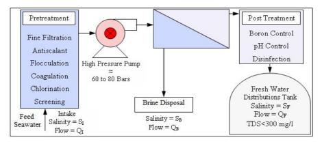
**Fig. 2.** A typical reverse osmosis seawater desalination plant scheme showing input/output and different stages of treatment. Note that boron control involves a second RO stage (BWRO), which also produces brine with a low TDS (<3000mg/l)
